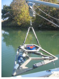
(b) Deployable ADCP sensor
