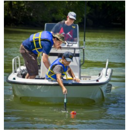
CITRIS, Berkeley Lab, and UC Berkeley's Department of Civil and Environmental Engineering and Department of Electrical Engineering unleash 100 floating sensors to understand how water flows through the Sacramento-San Joaquin Delta on its way to pumping stations and San Francisco Bay. Photo by Roy Kaltschmidt (Berkeley Lab).
