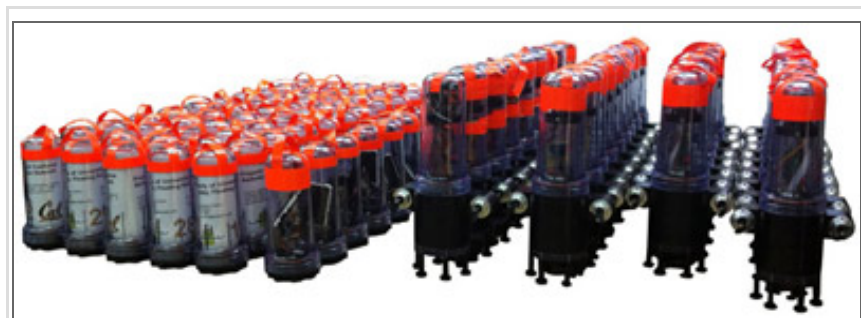
The floating robots on the left are passive, going where the currents take them. The devices on the right are autonomous and have propellers that help them maneuver away from obstacles in the water. (Jonathan Beard photo)
